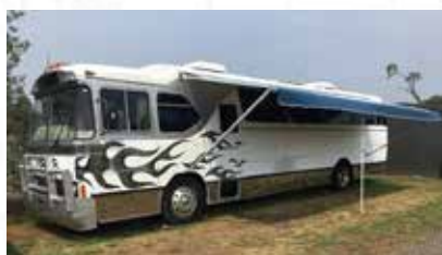
1978 PMC COACH 3208 Cat motor with 9 speed Roadranger gearbox, Rear airbag suspension, Caterpillar and Western star running gear throughout. Plus much more! DIY941938
